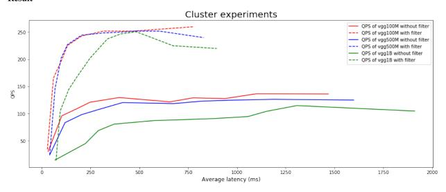
The growth shape of QPS is more like inverted J-shaped curve which means the growth of QPS basically have no obvious change when average latency exceed one certain number.
