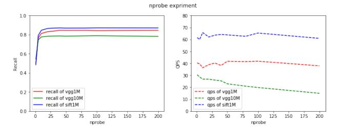
As we can see, when nprobe exceeds 25, there is no obvious change of recalls. Also, when nprobe get larger, only QPS of vgg10M get smaller, QPS of vgg1M and QPS of sift1M basically have no changes.
